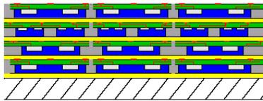
10 - Dicing street edges plating parallel process (electroless Ni + Au)
